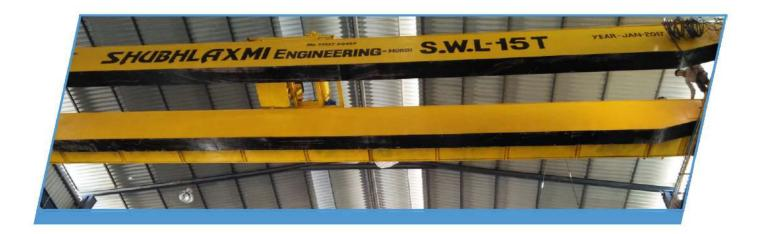
Shubhlaxmi Cranes make Double Girder EOT (Electric Overhead Traveling) Crane is Specially designed structures with mechanical means for Traveling in both directions and raising and lowering a load by electrical, and its consists of Structures, Wheels, Gearboxes, Wire Rope, Electrical Motors and Panels, Hook assembly etc. We recommend you the perfect customized solutions after doing an in-depth analysis of your applications.
