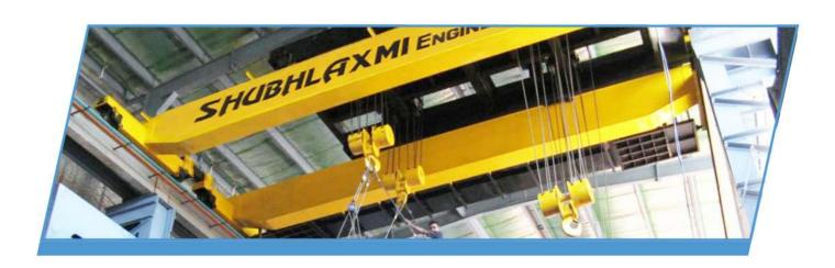
These under slung / Suspension Cranes are used in the areas where there is no option of the supporting steelwork beneath the floor. The track for such cranes is held by the roof structure or by the pillars. These cranes required less space and run on the lower flange of the crane runway. This flange is placed directly on the ceiling and is highly profitable in terms of judicious use of space. We manufacture these in compliance with the requisite industry standards.
