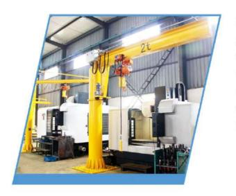
Shubhlaxmi Cranotech LLP Pillar mounted (Free Standing) Jib Cranes are best suited for work station application. These cranes are directly installed on shop floor without any need for support from building column. Available in capacity ranging from 0.5 MT to 5 MT and outreach of 8 meters, these cranes serve the need of local station without use of shop EOT Crane.
